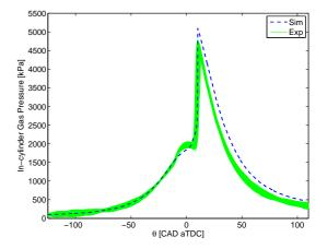
Figure 1: Comparing simulated and experimental pressure traces for test point #14 in Table 2.
